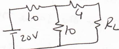
$$\text{Value of } R_L \Rightarrow \boxed{\frac{10}{10+4}} \quad R_L = R_i = 9\Omega$$
