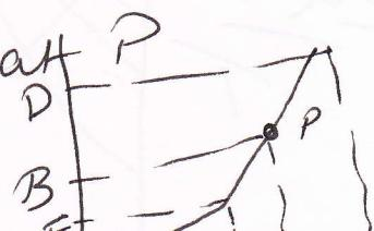
(ii) AC resistance - The opposition to the changing current flow in forward dir. is called ac. forward current resistance. It is ratio of change in voltage across diode to the change in current through it. ⑥
