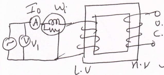
The circuit is as shown in figure. The supply V is increased to rated voltage  $V_1$  & reading of ammeter ( $I_0$ ) & wattmeter ( $W_i$ ) is noted down. As secondary is O.C., the primary current carries only no-load current  $I_0$  which is just 4-5% of Full load current of the transformer.  $\therefore$  Cu loss is very less (negligible) & primary winding is very less (negligible) & as Voltage is rated voltage, flux is rated &  $\therefore$  Core loss measured by is rated core loss.
