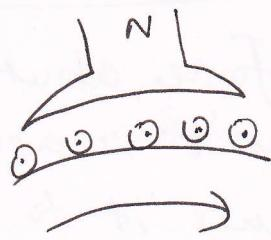
when electrical supply is given to the motor, with the interaction of armature current with main flux, a torque is produced & motor starts rotating in clockwise direction as given by Fleming's left hand rule
