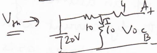
$$P_{max} = \frac{V^2}{4R_L} = \frac{100}{4 \times 9} = 2.78 \text{ W}$$
