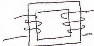
Transformers basically consist of 2 parts  $\equiv$  Cone winding
