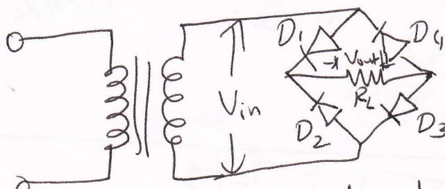
(i) Ripple factor =  $\frac{\text{rms. value of ac. comp.}}{\text{value of dc. comp.}}$
